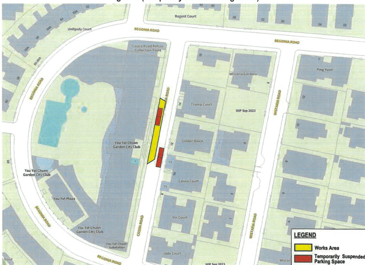
Figure 1 (Temporary Traffic Arrangement)
